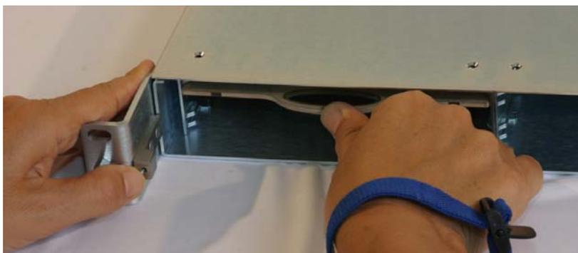
12. Place the front panel in its place on the chassis.
